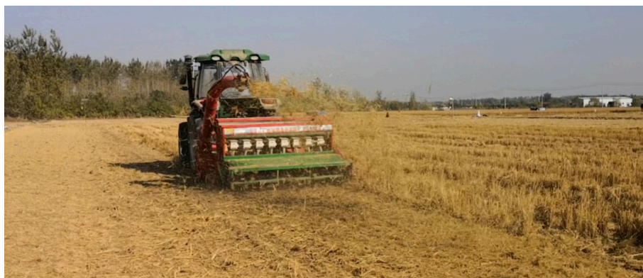
▲ Overall straw-barrier removal and fine-coverage seeding technology and equipment of straw-returning machine
